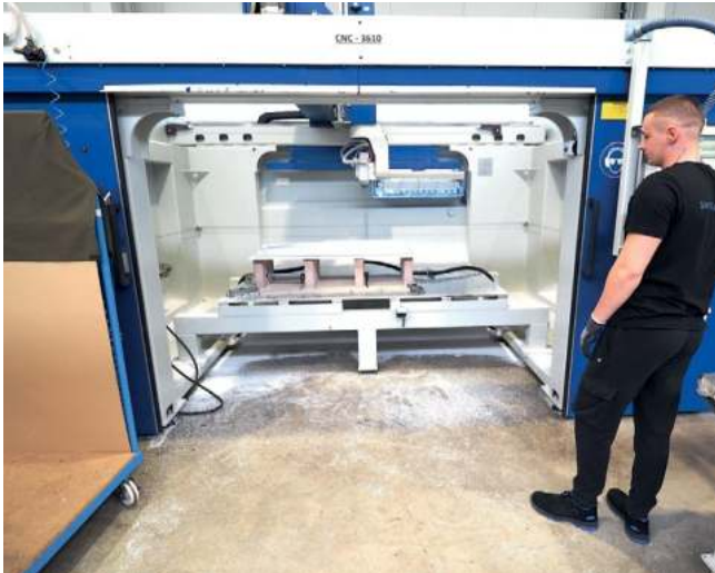
The 5-axis CNC machining center G-S-F(24-13)/B in gantry design was added in 2020
