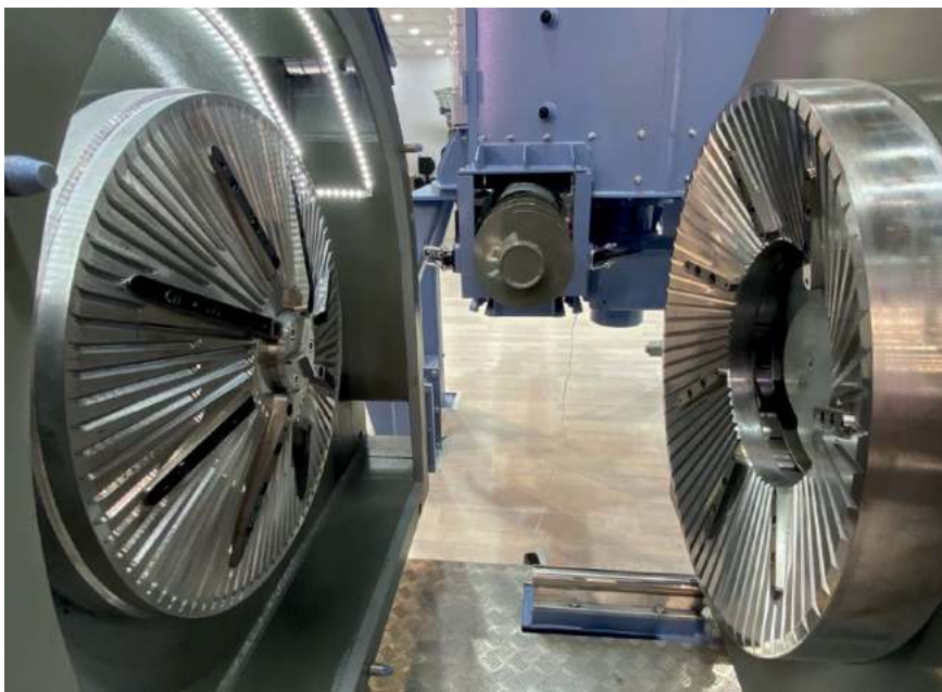
Plastcompactors process the feedstock in continuous operation between a rotating and a stationary disk
