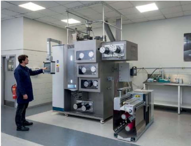
Multifilament plant at the FET Fiber Development Center (©FET)
