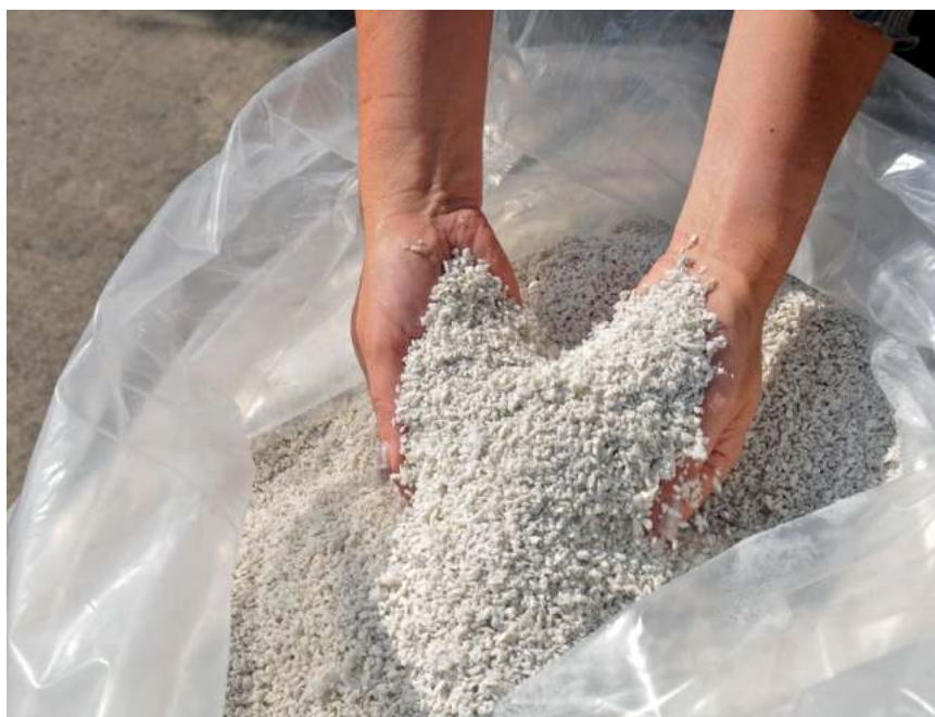
The agglomeration produces a free-flowing regrind of high bulk density
