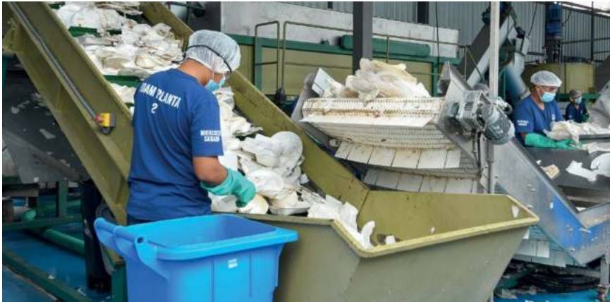
Sorting polystyrene packaging from the post-consumer sector
