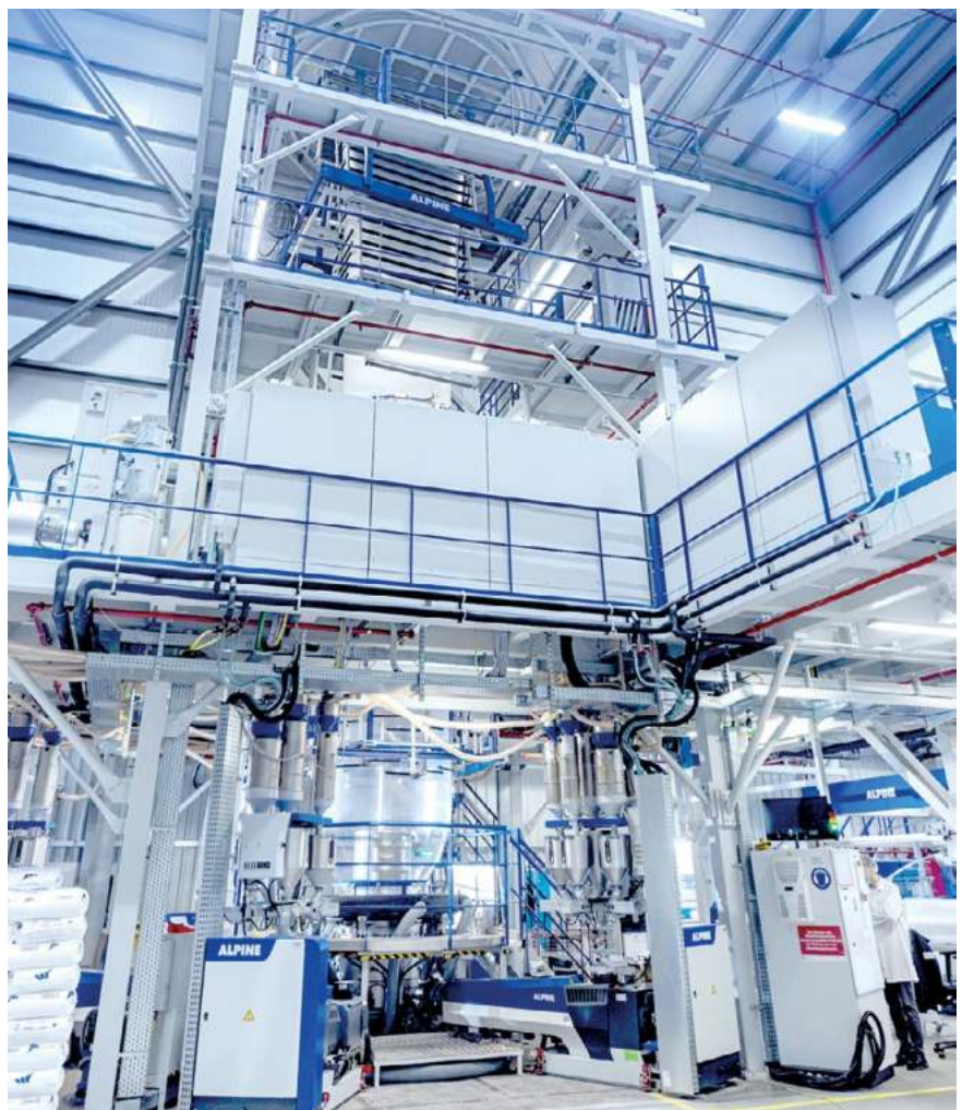
The modern 5-layer blown film line with inline MDO at Constantia Flexibles in Pirk has twelve rollers. This improves the homogeneity of the stretched film as it has more time to cool down after stretching
