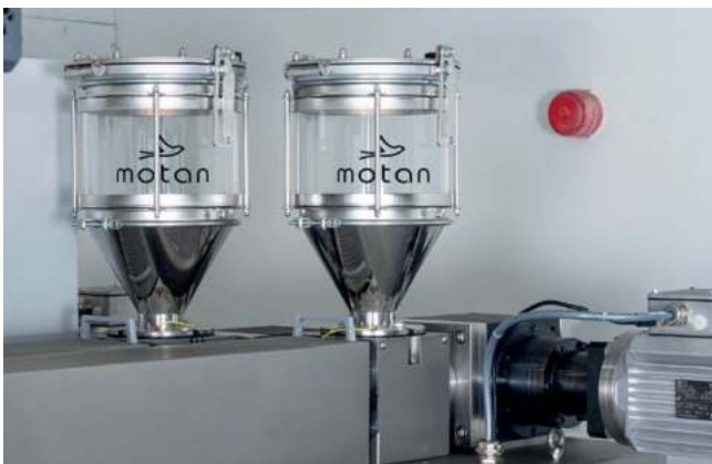
motan glass machine hopper for holding specially modified glass containers with dried material (©FET)
