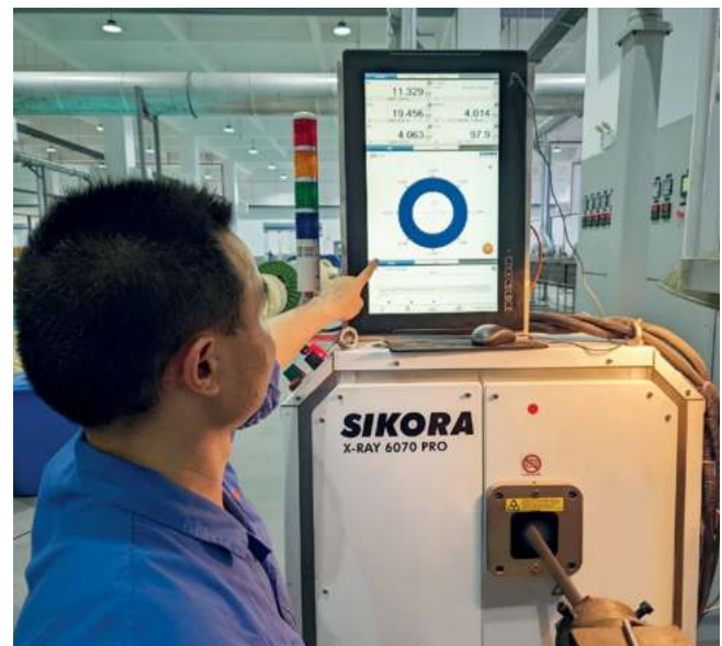
Wuxi Huacheng Cable uses SIKORA's X-RAY 6000 PRO for measuring and control during new energy cable production
