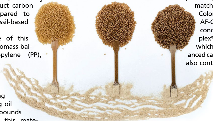
Three M-BIOBASE® compounds with different proportions of wood fibres (© BIO-FED)
