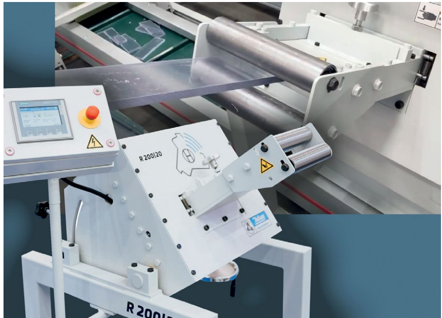
The touchscreen on Hellweg's R 200/20 edge trimming system, which is equipped with a servo geared motor, allows cycle times to be freely set. This means that the size and number of individual chips can be optimized for further processing independently of extrusion system output (© Hellweg Maschinenbau)
